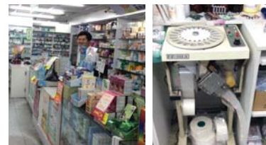
The pharmacist happily smiling is the son of Mr Joseph Wang who has a whole family (his wife, and daughter in law) all working as pharmacist! Depending on patients' needs, the drugs for the same administration time can be packed together in a unit packet using the machine as shown.
